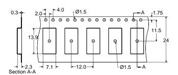
Dimensions shown are nominal in millimeters Packaging quantity: 2000 units/reel
